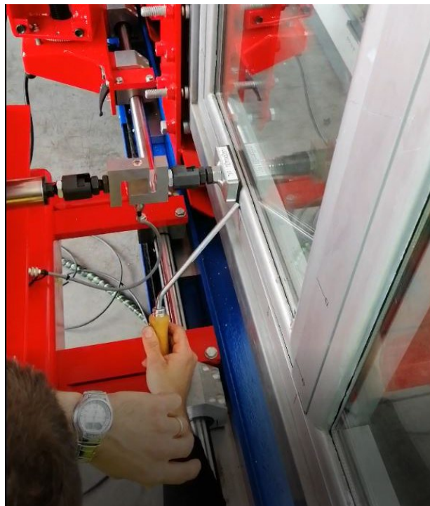
FIGURE 1 PICTURE SHOWING A STATIC ATTACK TEST FOR RC2 OR RC3 TEST
