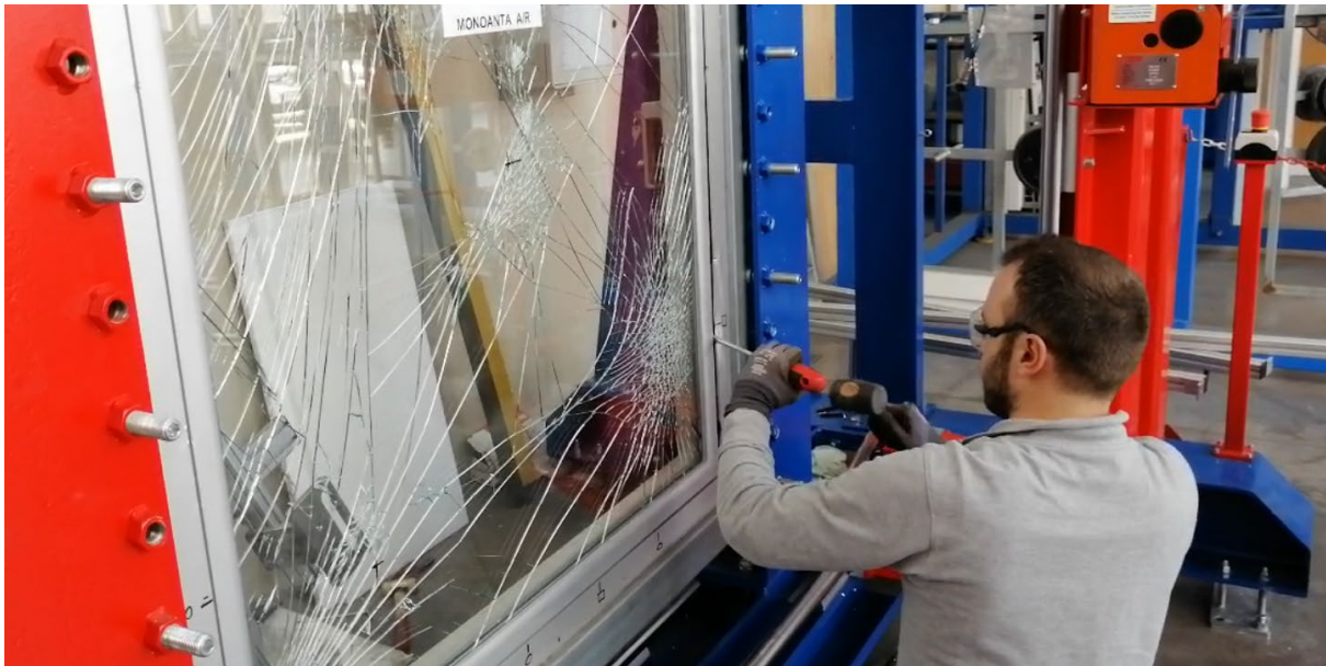
FIGURE 2 PICTURE SHOWING A MANUAL ATTACK TEST FOR RC2 OR RC3 TESTS
